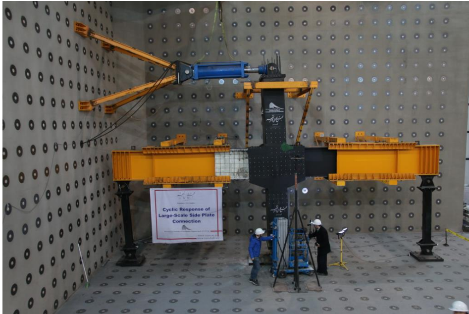
Figure 1.2. Extensive laboratory resources are required for large-scale structural tests: A steel beam-to-column connection tested by the International Institute of Earthquake Engineering and Seismology [11].
